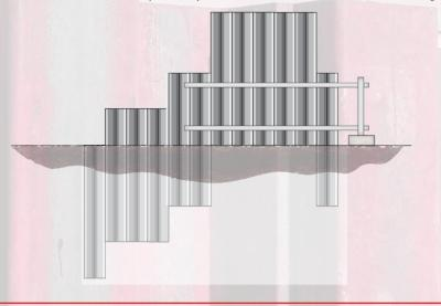
First panel completed, second panel part driven, third panel pitched. The last pair of the second panel becomes the first pair of the third panel.
