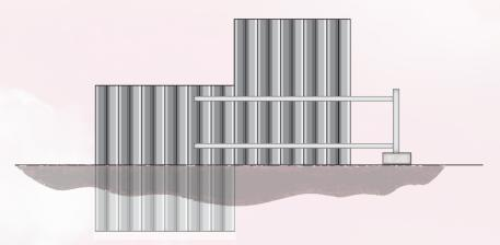
First panel driven to final level in stages. The last pair of the second panel plumbed and driven accurately.
